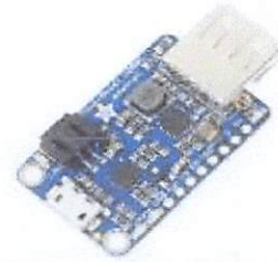
Figure 11. Power Boost Rechargeable
